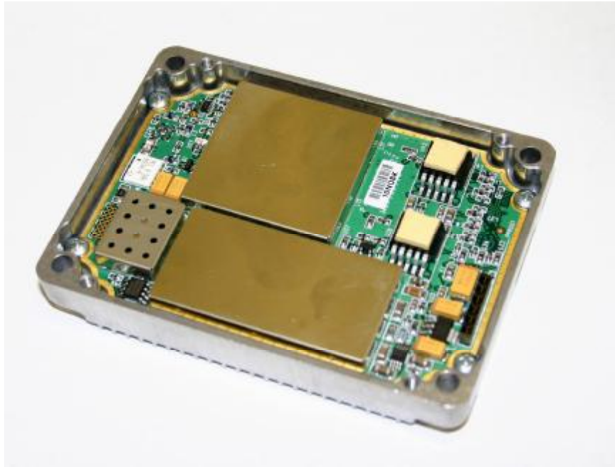
Photo 1: Internal with shielding
