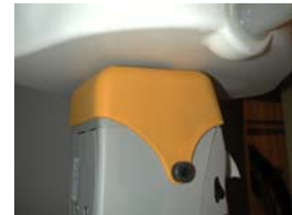
Figure 14.13 Body SAR Test Setup -- w/o Holster --
