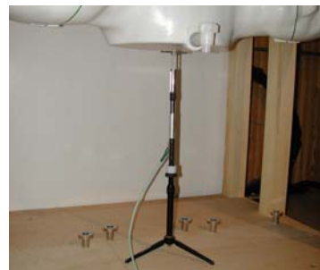
Figure 12.1 Dipole Validation Test Setup
