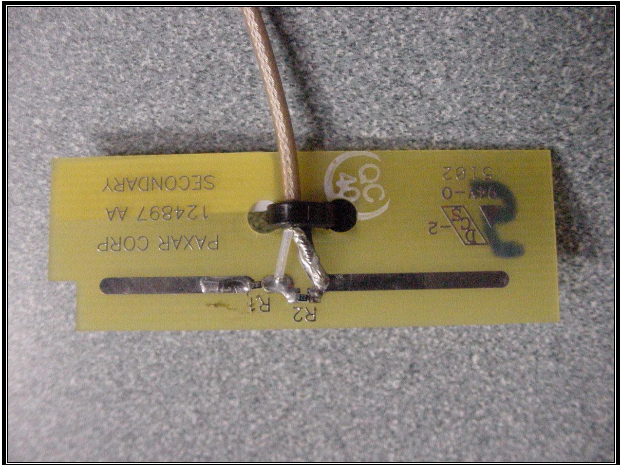
PHOTOGRAPH 27: FRONT OF ANTENNA
