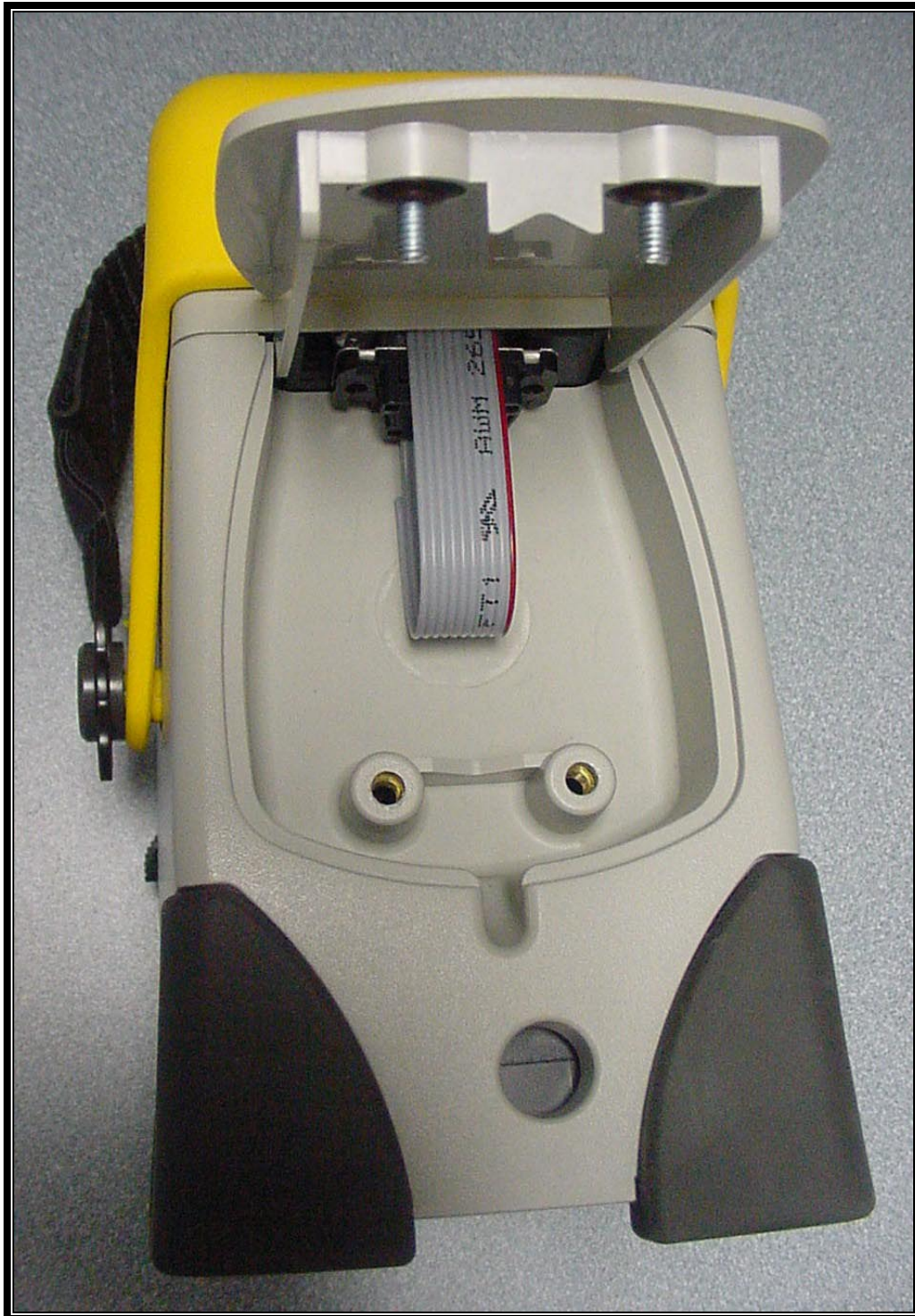
PHOTOGRAPH 11: EUT BACK COVER OPEN SHOWING DATA CABLE
