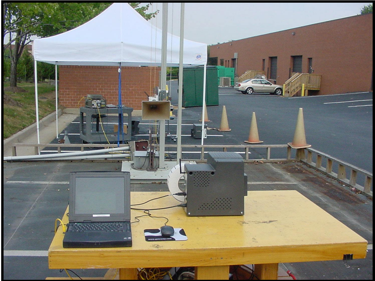
PHOTOGRAPH 6: RADIATED EMISSIONS FRONT VIEW; WORST CASE CONFIGURATION
