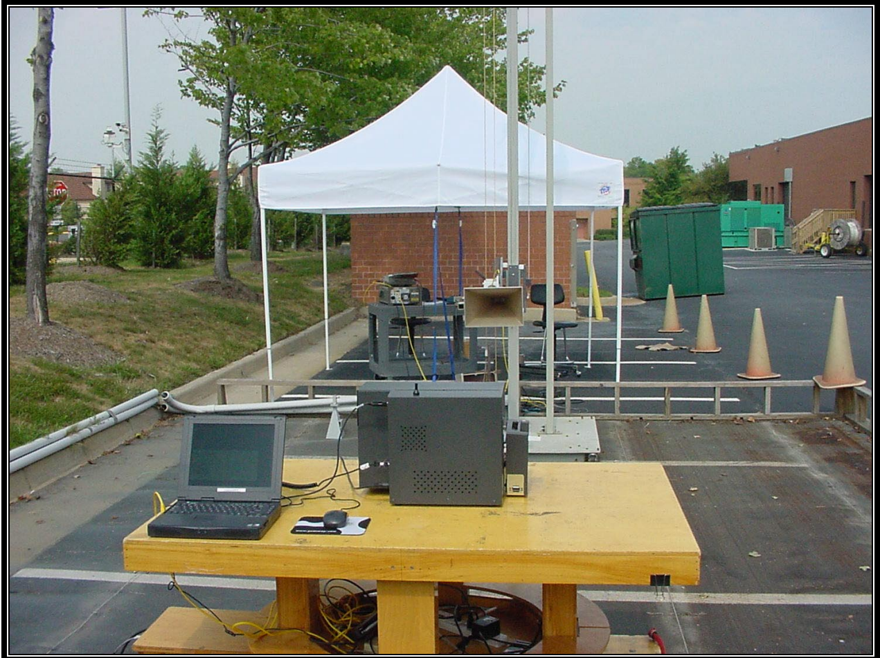
PHOTOGRAPH 10: RADIATED EMISSIONS FRONT VIEW; WORST CASE CONFIGURATION
