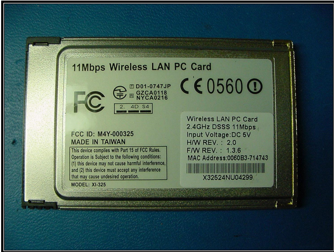
PHOTOGRAPH 23: WLAN CARD REAR VIEW
