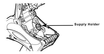
**3.** Place the supply roll in the supply holder so the supply feeds labels from the bottom.
