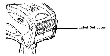
**3.** Feed all four inches of the backing paper **under** the applicator roller, **over** the peel bar, and **under** the label deflector.
