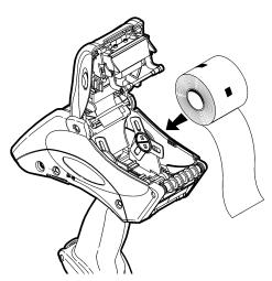
**4.** Load the supplies for the print mode you want. See "Loading for Peel Mode" or "Loading for Non-Peel Mode" for more information.
