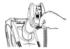
3. Take the thin end of the safety strap, and push it through the loop at the bottom of the printer handle (near the battery compartment).
