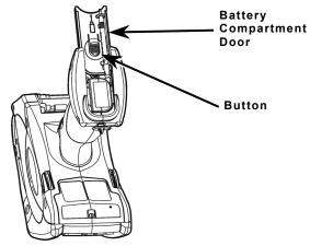
2. Turn the printer upright, holding your palm beneath the open battery compartment. Hit the printer on your hand and catch the battery as it slides out.
