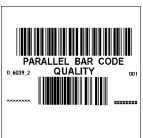
A label prints with barcodes to scan to check the quality of parallel bar codes
