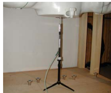
Figure 12.1 Dipole Validation Test Setup
