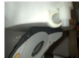
Figure 14.1 Body SAR Test Setup -- w/o Holster --
