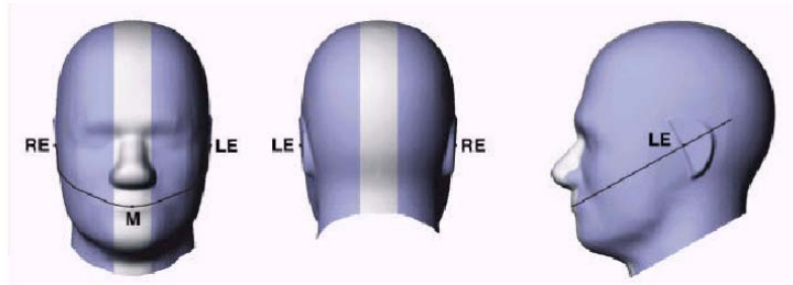
Figure 8.1 Front, back and side view of SAM Twin Phantom
