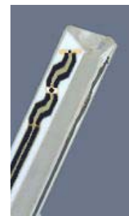
Figure 3.2 Probe Thick-Film Technique
