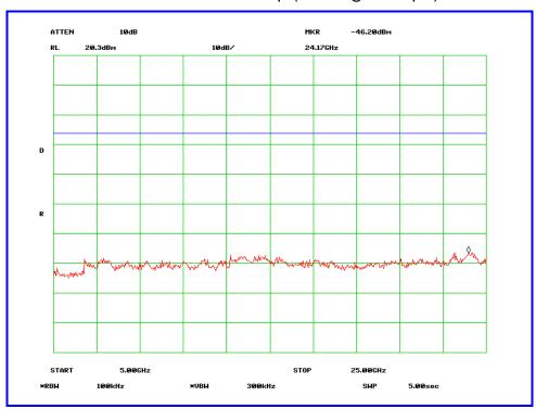
High Channel - Data Rate: 1 Mbps (Emission @ Antenna port)
