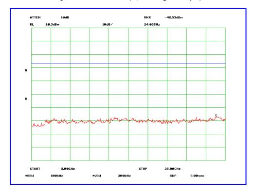
Low Channel - Data Rate: 2 Mbps (Emission @ Antenna Port)
