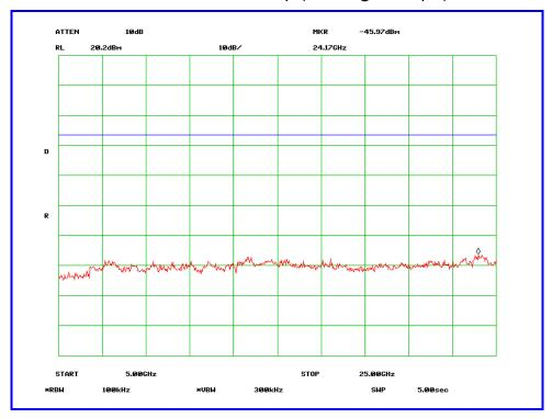
High Channel - Data Rate: 2 Mbps (Emission @ Antenna port)
