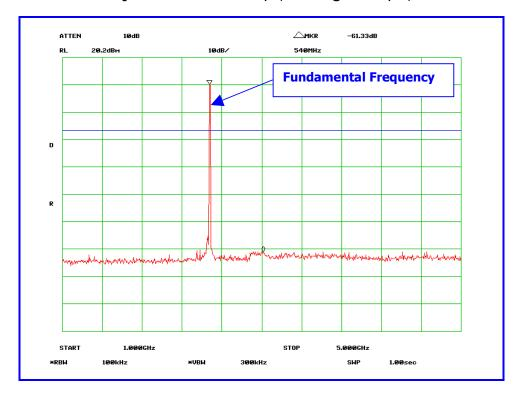
High Channel - Data Rate: 2 Mbps (Emission @ Antenna port)
