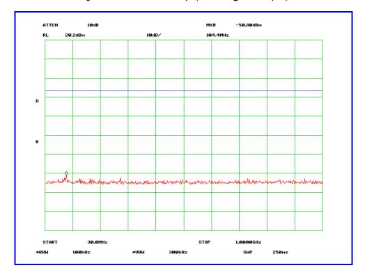
High Channel - Data Rate: 3 Mbps (Emission @ Antenna port)
