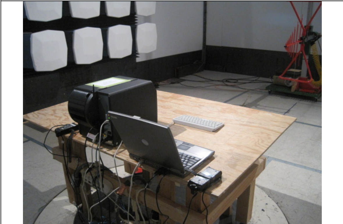
Host: 9906 Radiated Emission Test Setup – Rear View
