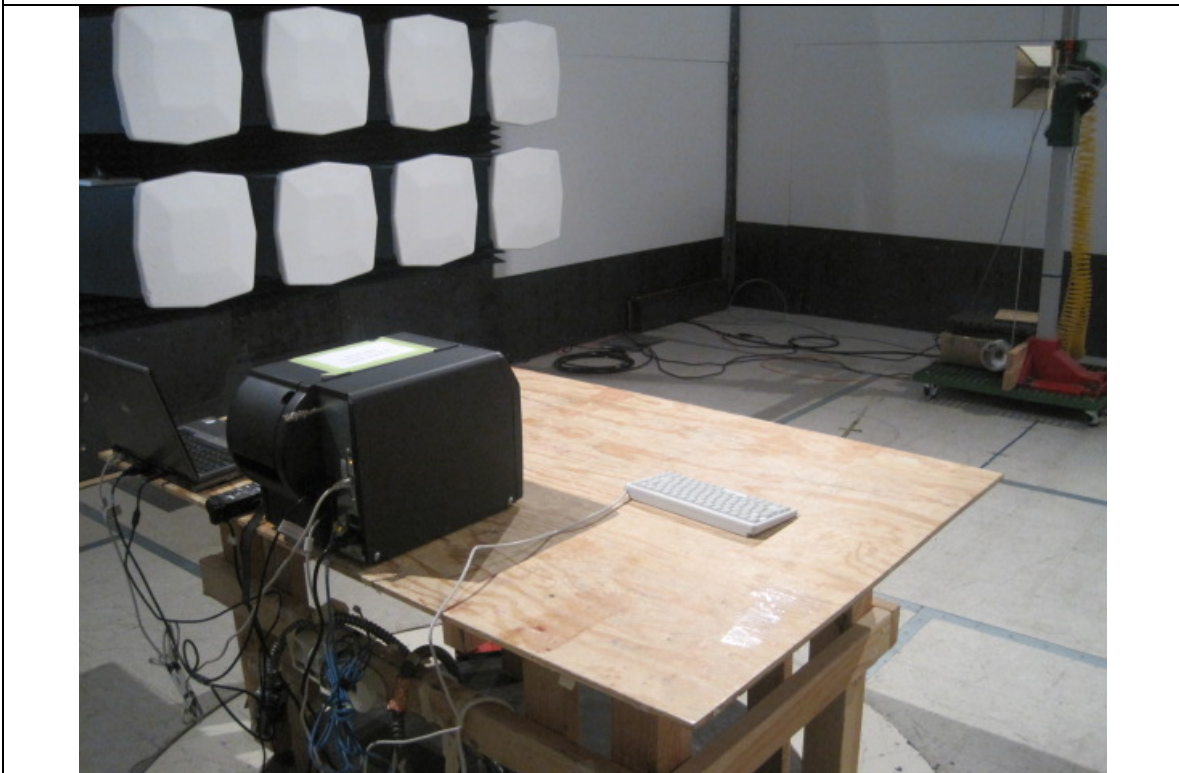
Host: 9906 Radiated Emission Test Setup – Rear View
