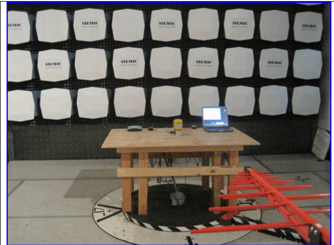
Host: 9460 Radiated Emission Test Setup – Front View
