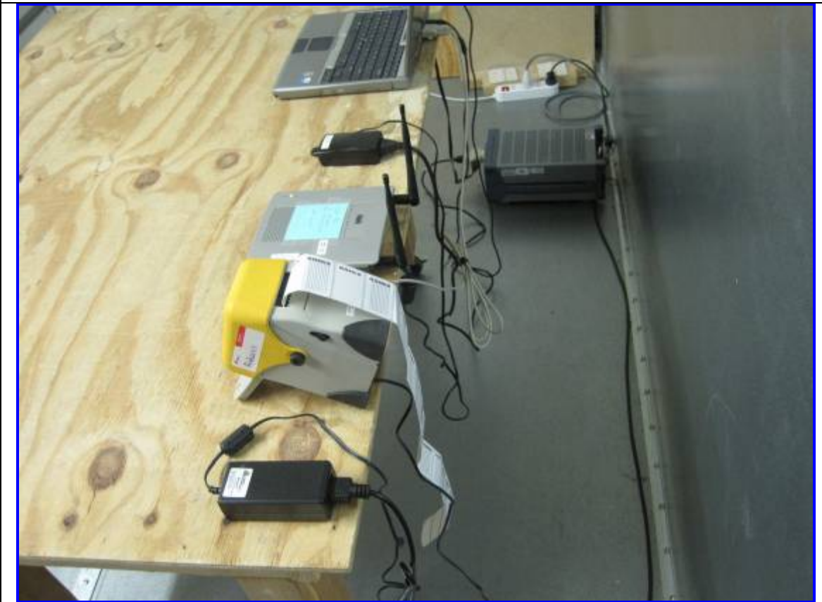
Host: 9460 Conducted Emission Test Setup – Rear View
