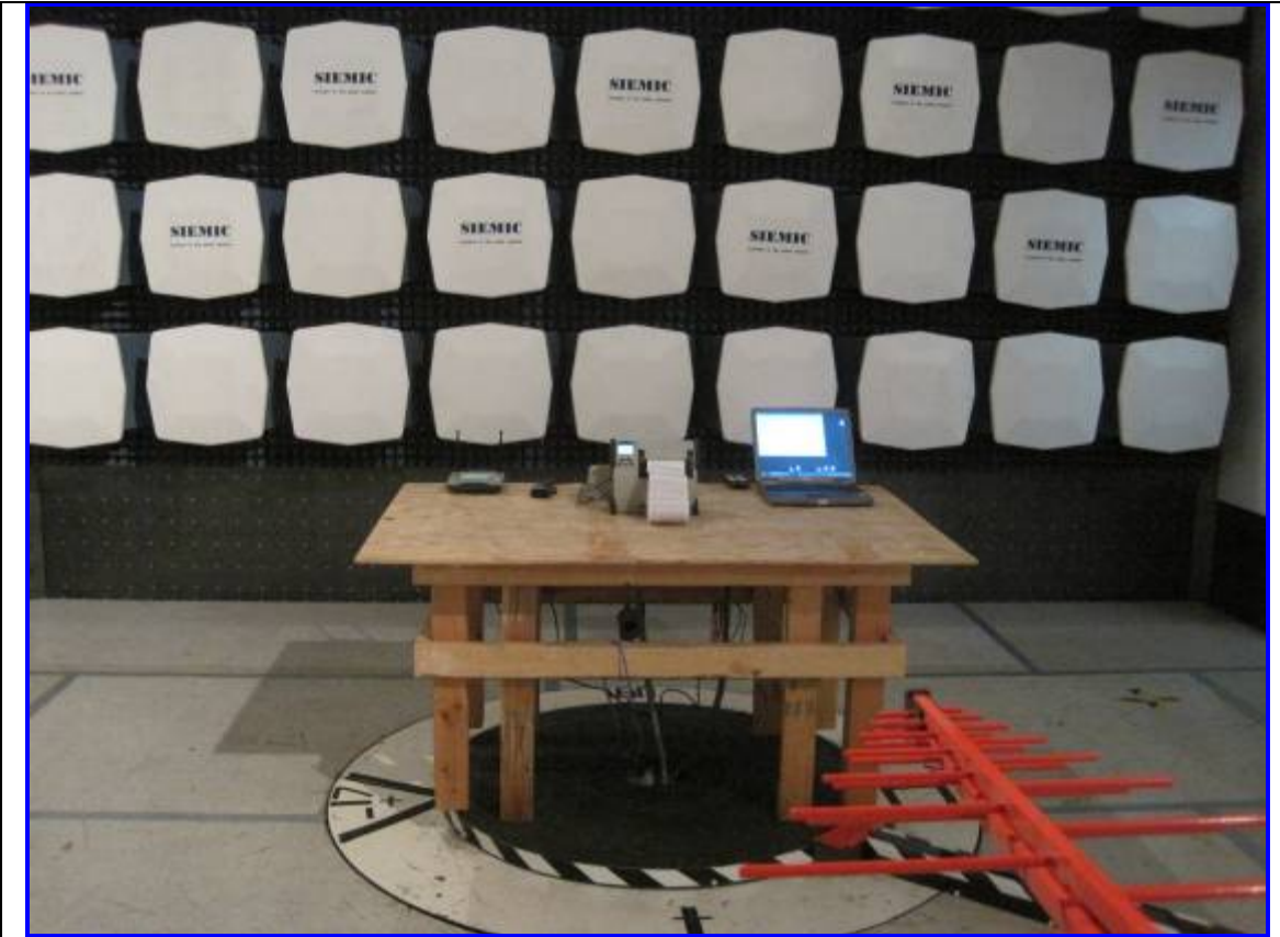
Host: 9493 Radiated Emission Test Setup – Front View
