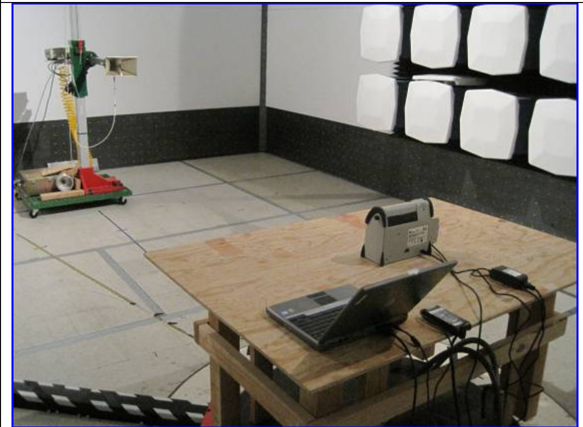
Host: 9493 Radiated Emission Test Setup – Rear View
