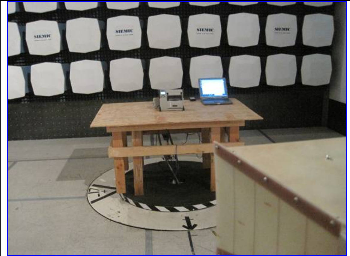
Host: 9493 Radiated Emission Test Setup – Front View
