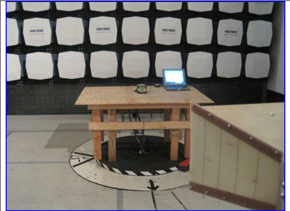
Host: 9433 Radiated Emission Test Setup – Front View
