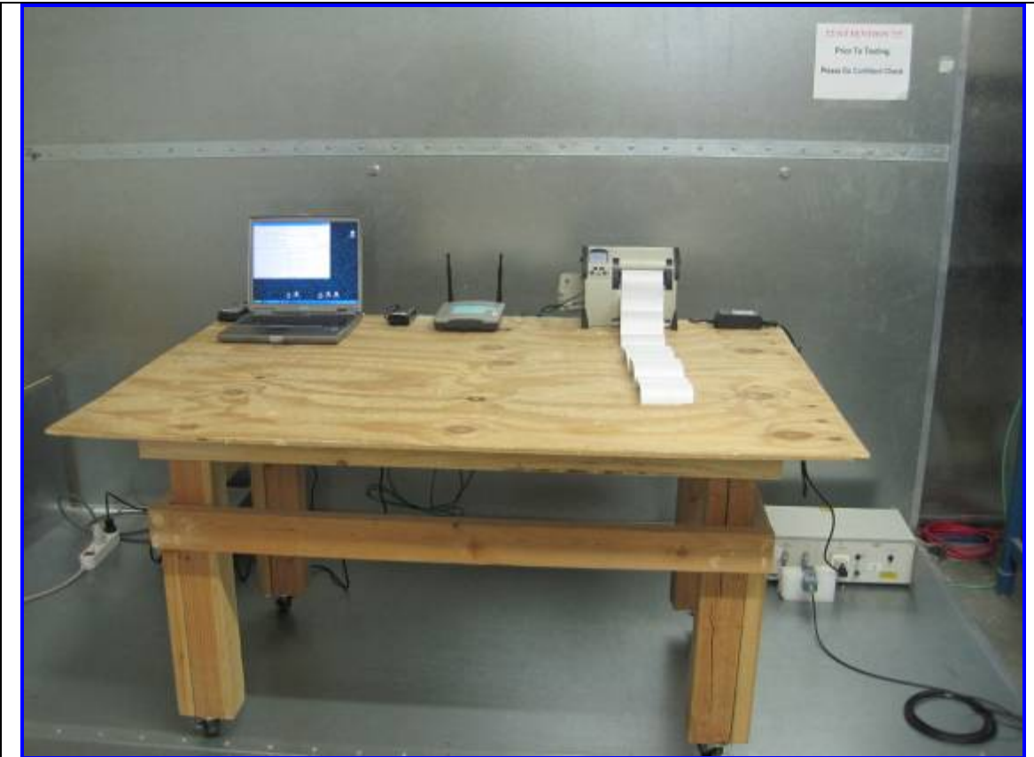
Host: 9493 Conducted Emission Test Setup – Front View
