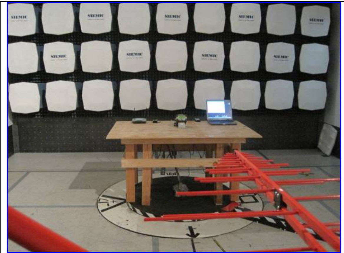
Host: 9433 Radiated Emission Test Setup – Front View
