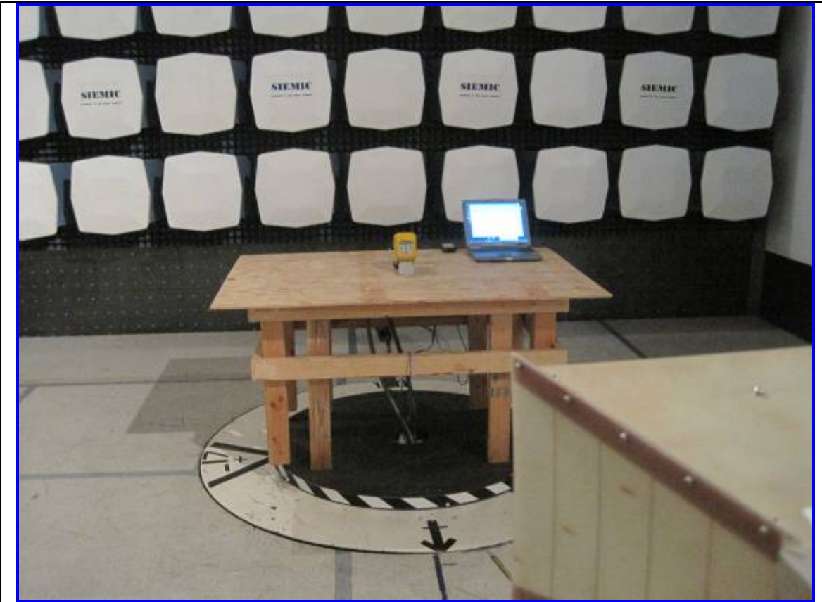
Host: 9460 Radiated Emission Test Setup – Front View
