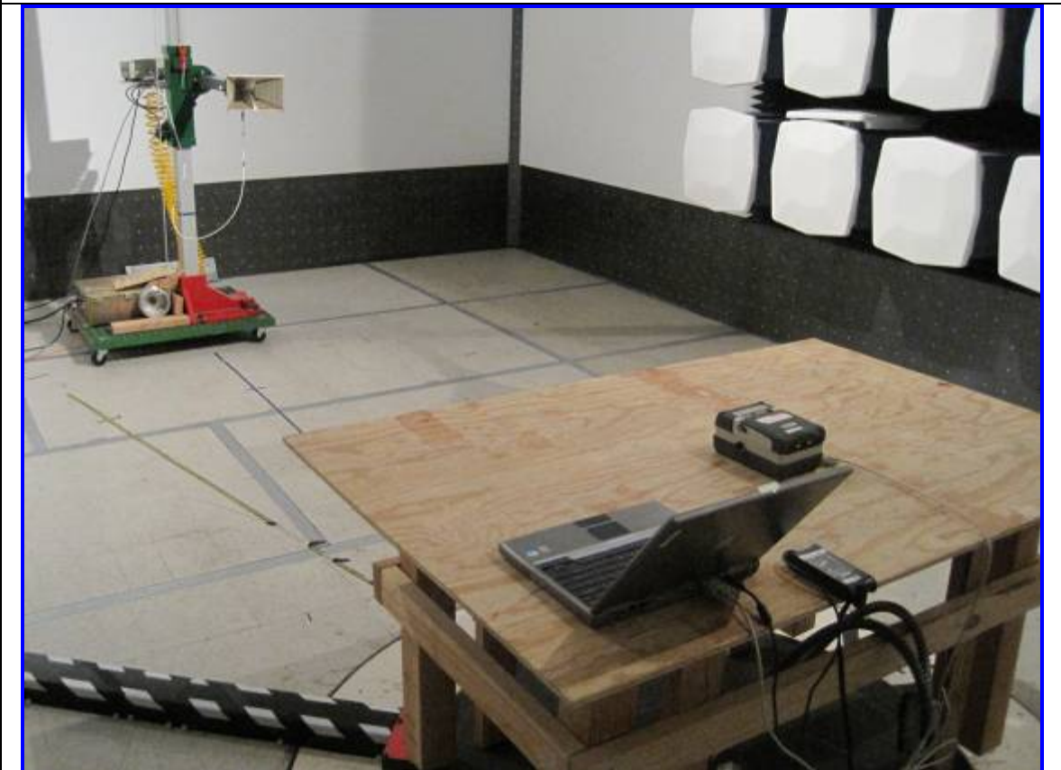
Host: 9433 Radiated Emission Test Setup – Rear View
