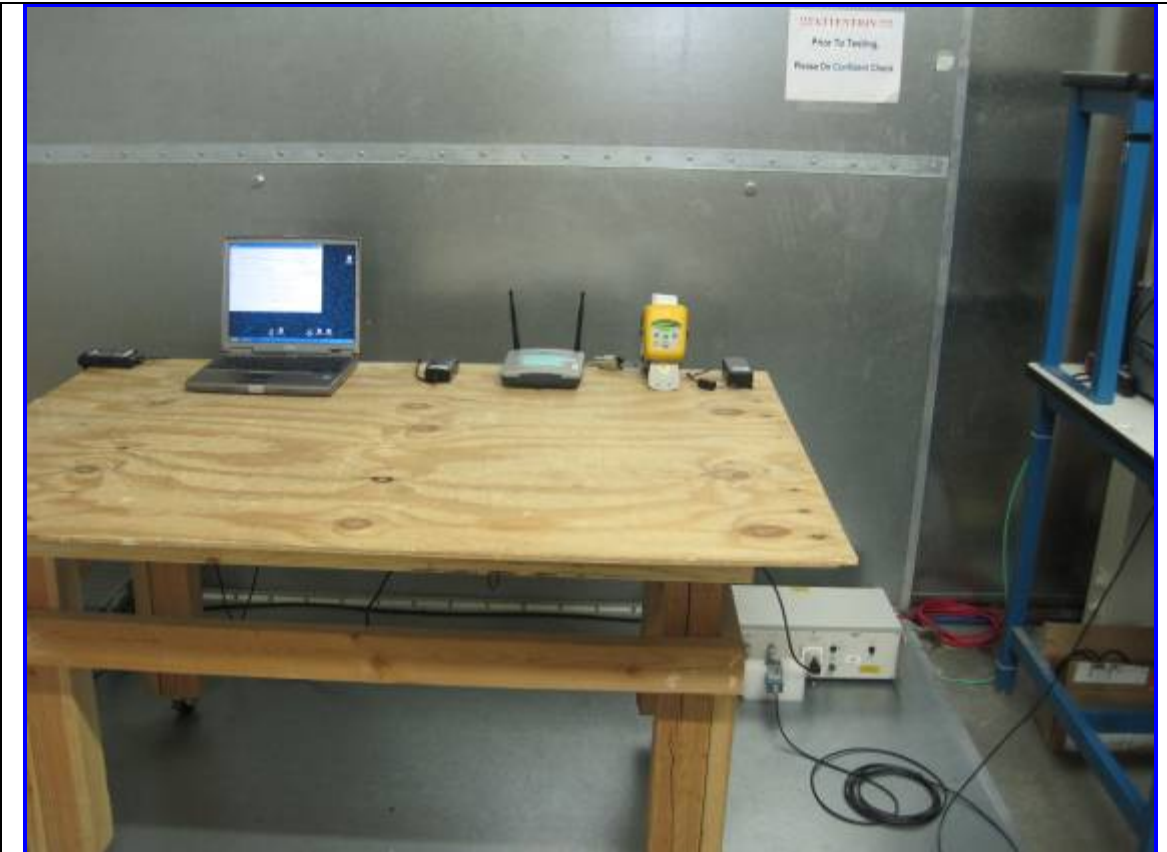
Host: 9460 Conducted Emission Test Setup – Front View
