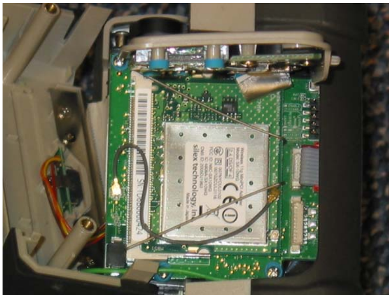
RF Module And Antenna
