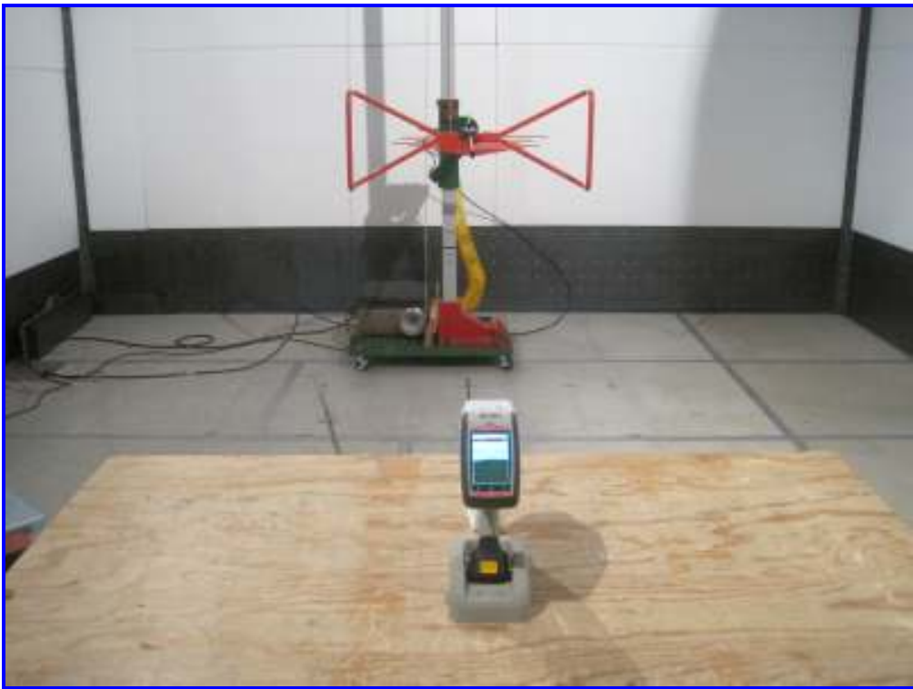
Radiated Emission, Host 6057 2D Scanner WiFi (30 MHz-1 GHz) – Rear View
