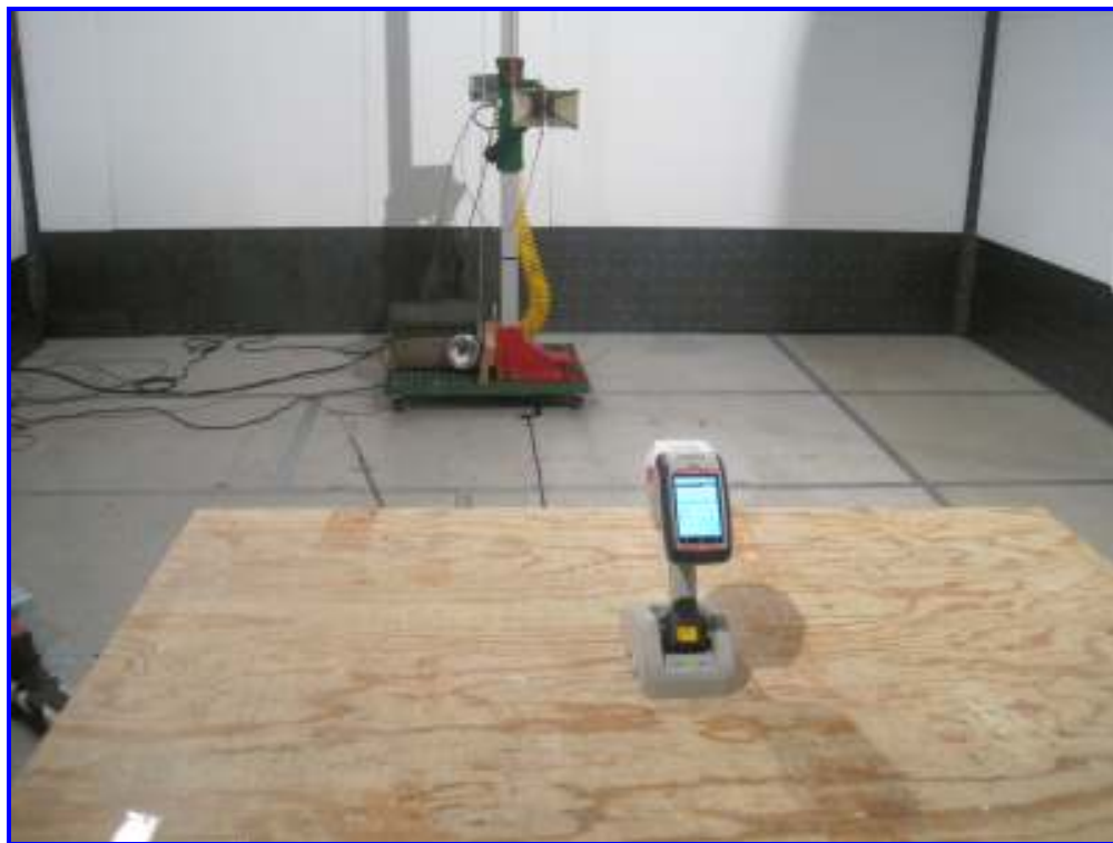
Radiated Emission, Host 2D Scanner WiFi (Above 1 GHz) – Rear View
