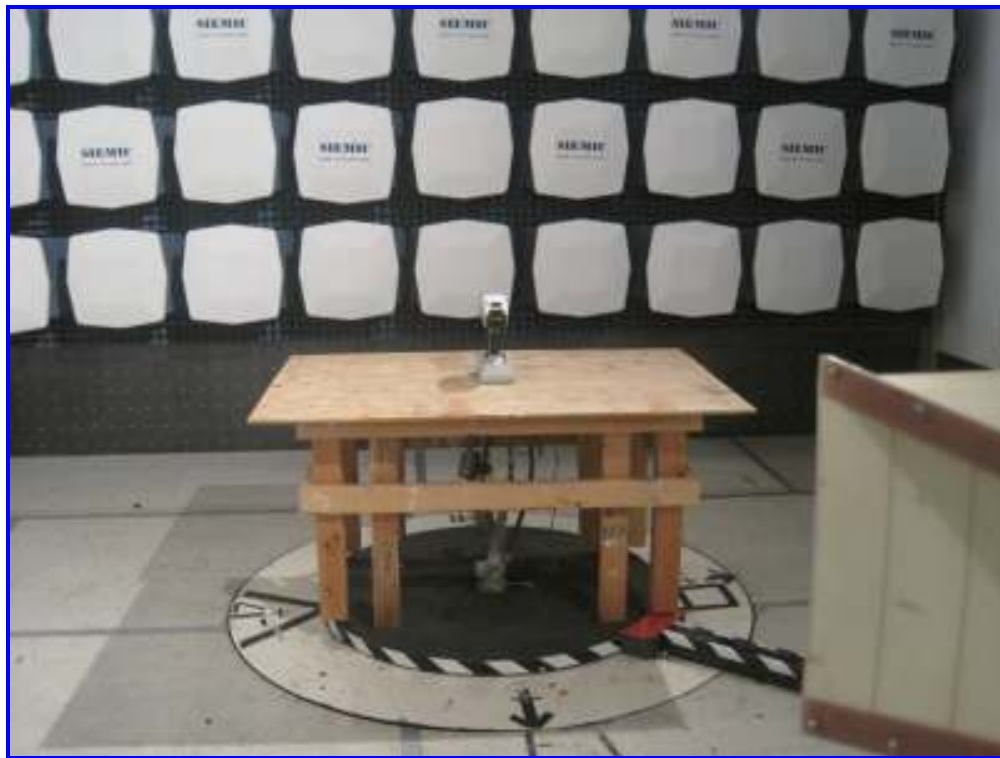
Radiated Emission, Host 2D Scanner WiFi (Above 1 GHz) – Front View
