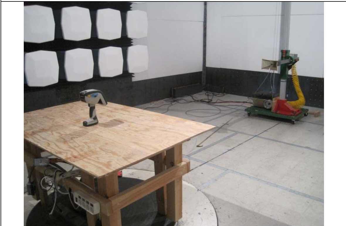
Radiated Emission Test Setup – Rear View
