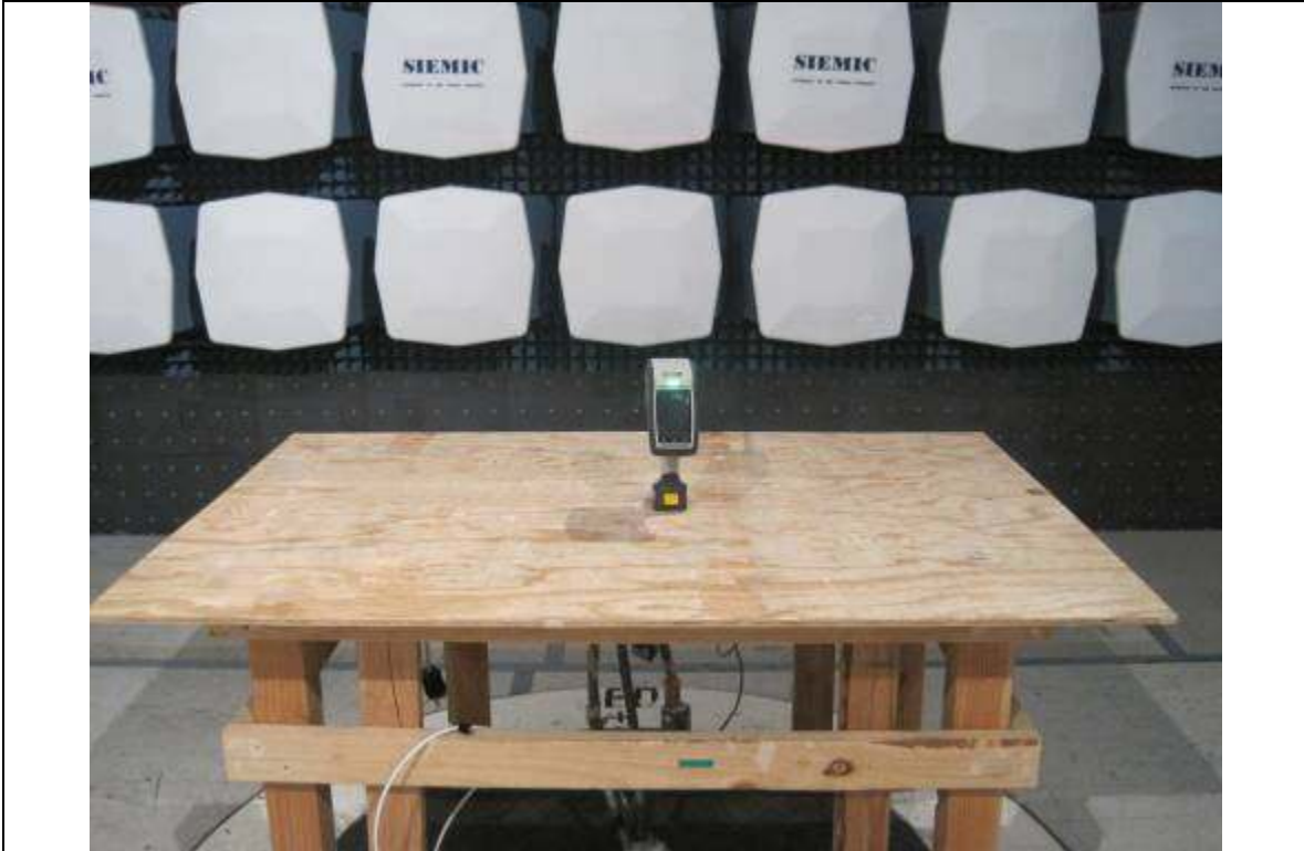
Radiated Emission Test Setup – Front View
