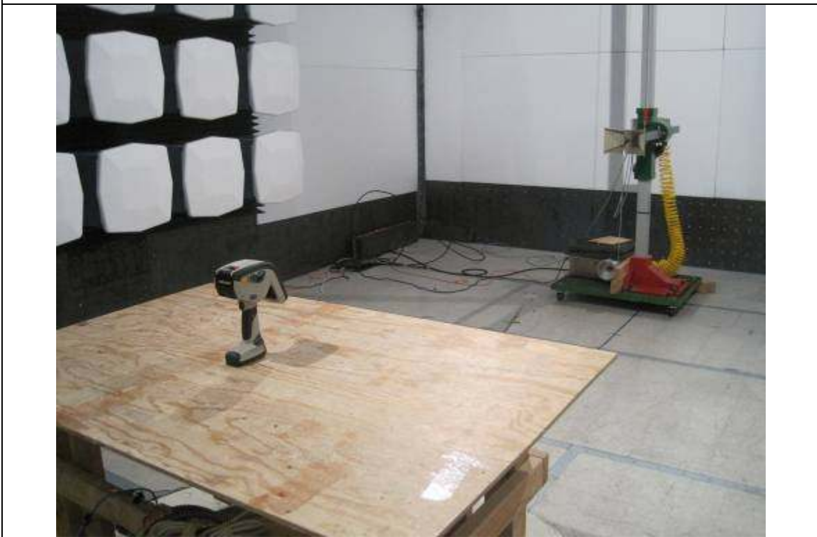
Radiated Emission Test Setup – Rear View
