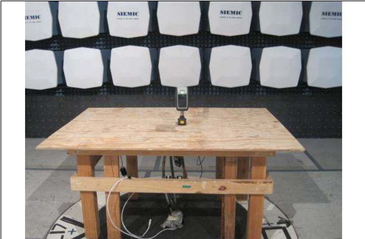
Radiated Emission Test Setup – Front View
