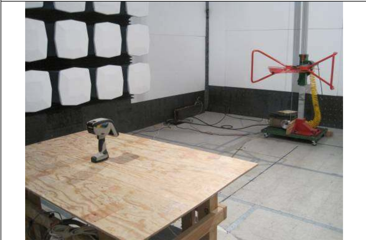
Radiated Emission Test Setup – Rear View
