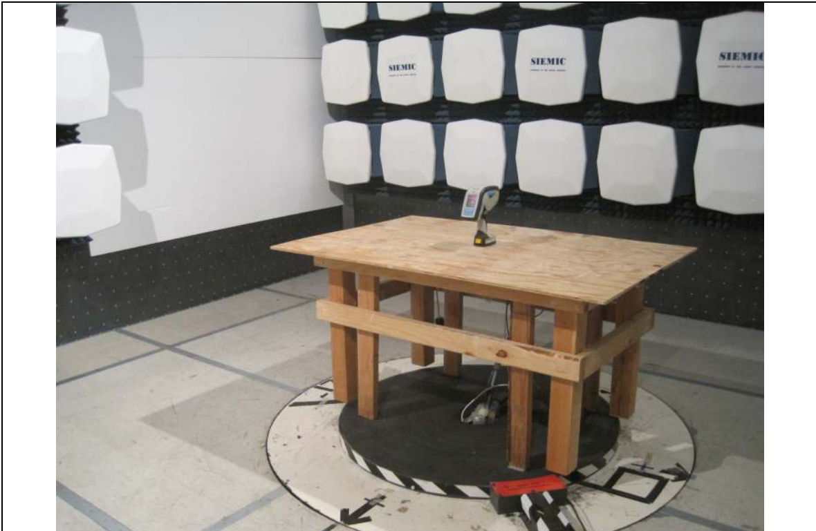
Radiated Emission Test Setup – Front View
