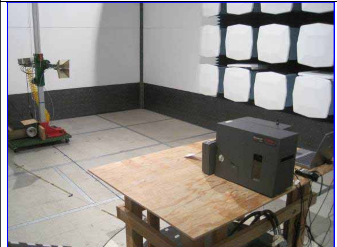
Host: 9855RFMP Radiated Emission Test Setup – Rear View
