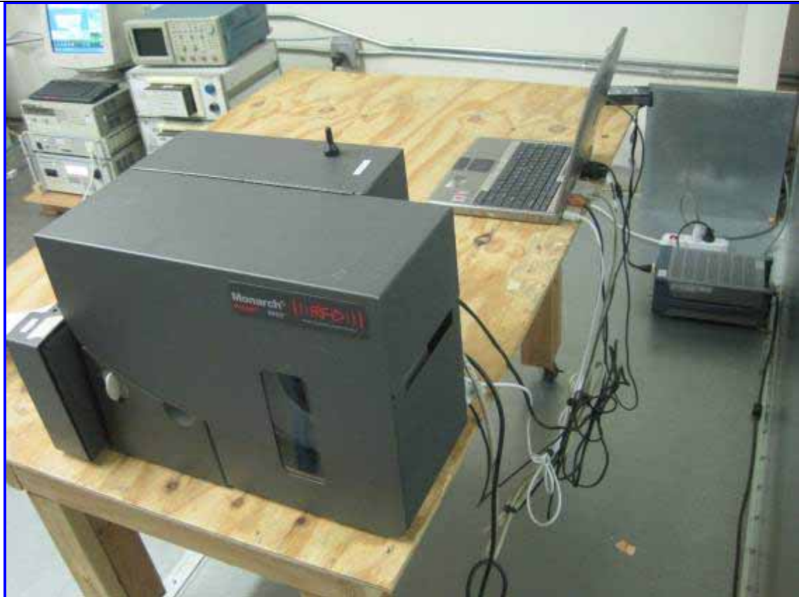
Host: 9855RFMP Conducted Emission Test Setup – Rear View
