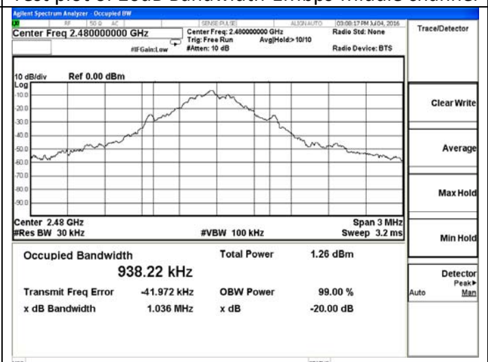
Test plot of 20dB Bandwidth-1Mbps-High channel
