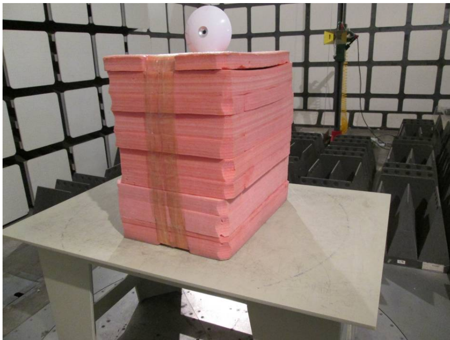
Radiated Emissions View (Above 1 GHz)
