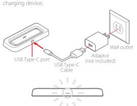
1. Insert the USB Type-C cable into the dock's USB port as shown 2. Place the speaker on the dock, the LED of the dock will light below and connect the other end to any USB adaptor or up white, indicating that the speaker is properly placed.
