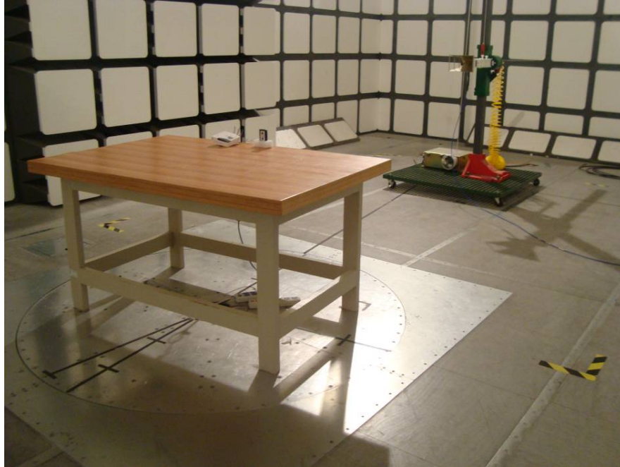
Above 1 GHz: Spurious Radiated Emissions - Front View
