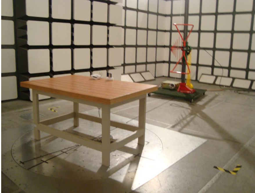
Below 1 GHz: Spurious Radiated Emissions - Front View
