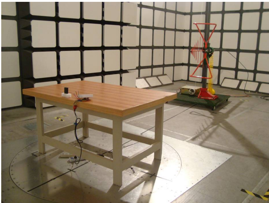
Below 1 GHz: Spurious Radiated Emissions - Rear View
