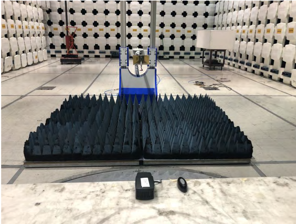
Radiated Emissions Test Setup, 1-13 GHz
