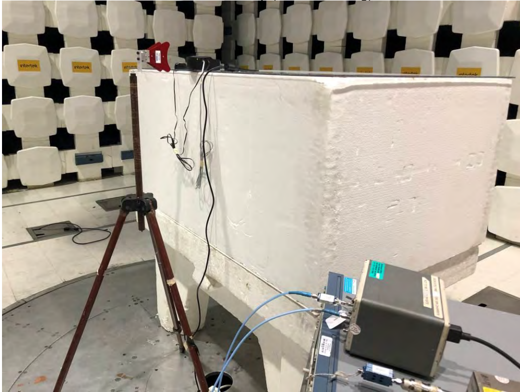
Radiated Emissions Test Setup (Manual Testing), 18-25 GHz
