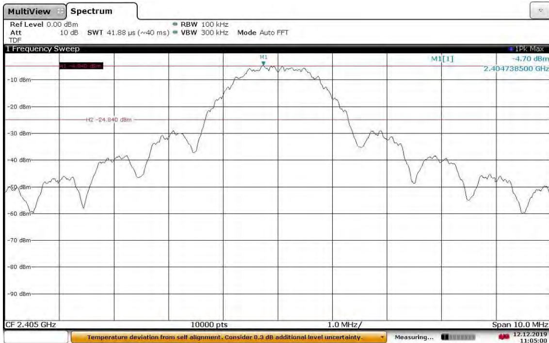
Antenna Port Conducted Emissions – Low Channel 20 dB Down From the Carrier Limit
