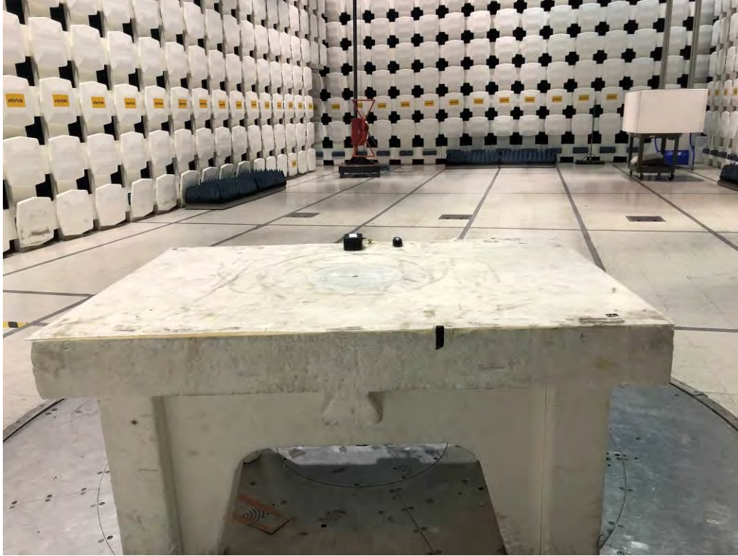
Radiated Emissions Test Setup, 30-1000 MHz
