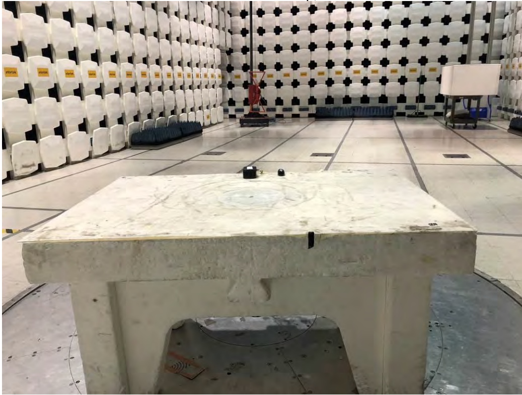
Radiated Emissions Test Setup, 30-1000 MHz
