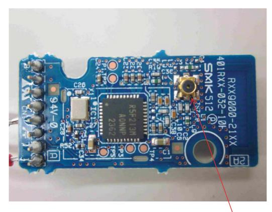
The antenna connector shown in this photo is used for testing only and is not provided in the mass production.
