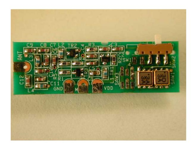
Fig. D-6 Bottom View of RF Unit
