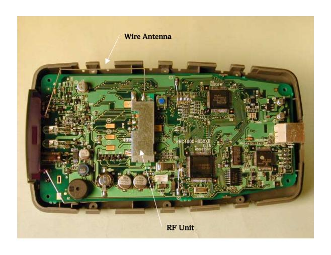
Fig. D-5 Top View of RF Unit
