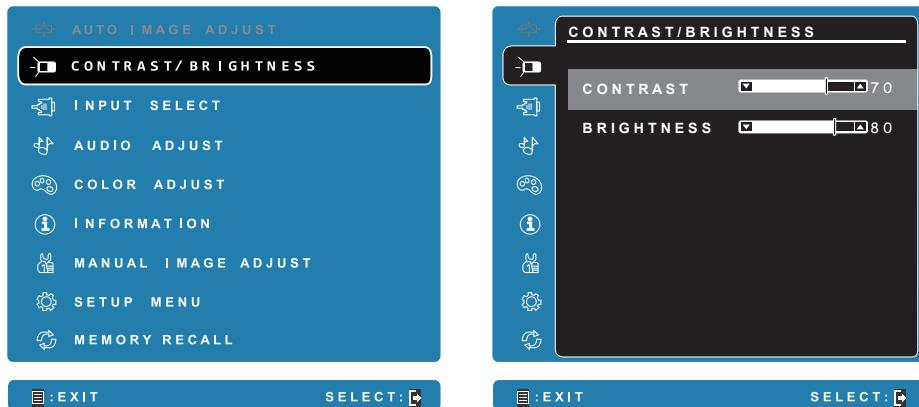
Press the **Menu/Exit** button on bottom right of your VSD243 to launch the OSD configuration screen. The OSD configuration screen can be used to configure the Contrast/Brightness, Input Select, Audio Adjust, Color Adjust, Information, Manual Image Adjust, Setup Menu and Memory Recall.
