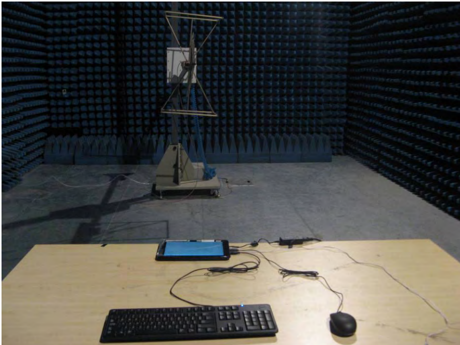
FCC RADIATED EMISSION TEST SETUP
