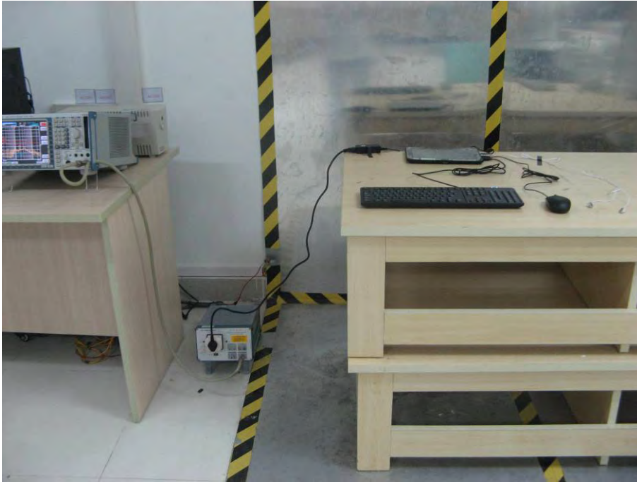
FCC LINE CONDUCTED EMISSION TEST SETUP
