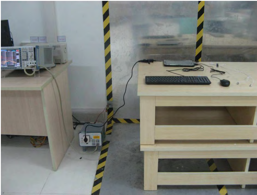
FCC LINE CONDUCTED EMISSION TEST SETUP
