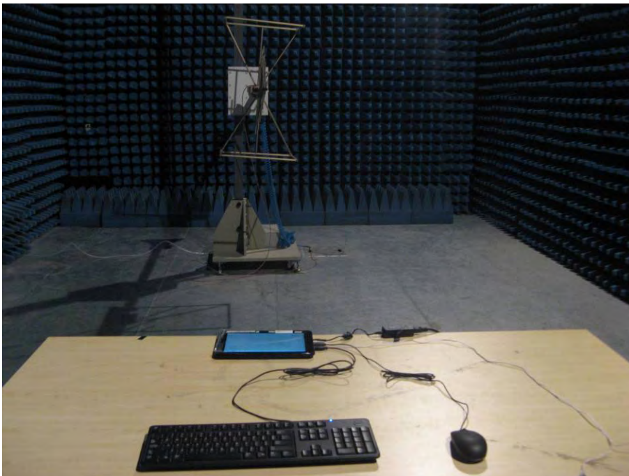
FCC RADIATED EMISSION TEST SETUP
