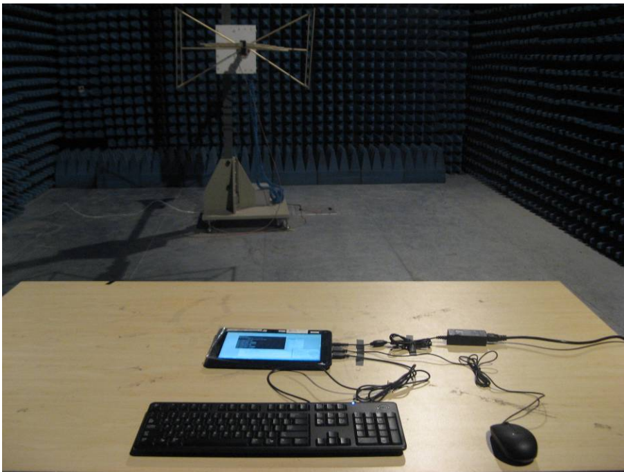
FCC RADIATED EMISSION TEST SETUP
