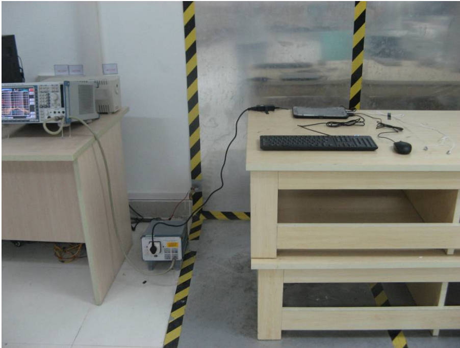
FCC LINE CONDUCTED EMISSION TEST SETUP
