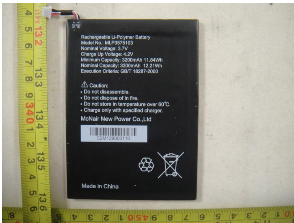
Battery (Model: MLP3575103, which is used for SAR measurement in this report)
