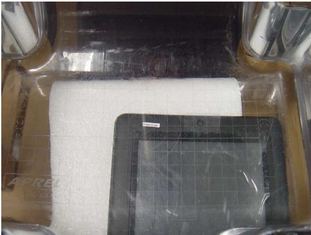
Figure B.2 EUT Frontside Towards phantom
