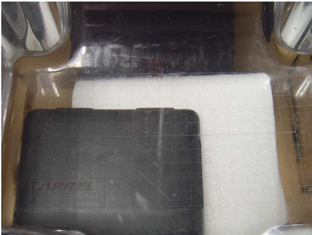
Figure B.3 EUT Backside Towards phantom
