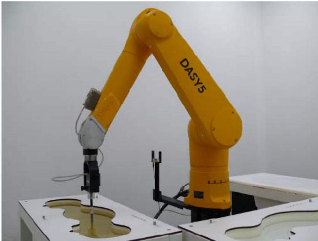
Picture 1: Specific Absorption Rate Test Layout
