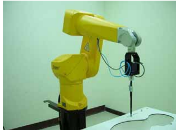
Fig. 5.2 Probe setup on robot
