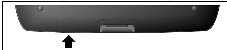
Figure 11: The Auxiliary Battery Port
