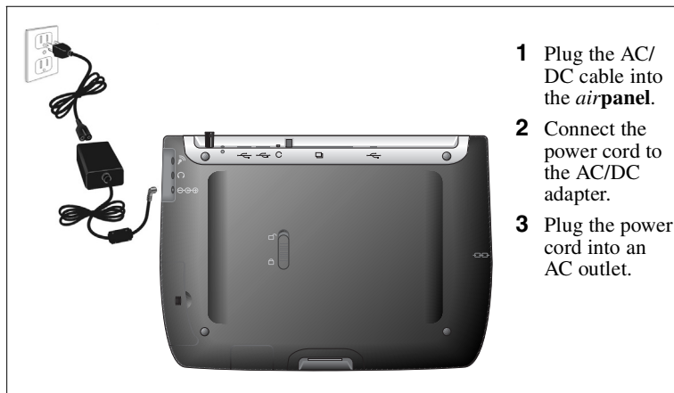
Figure 4: Using the AC/DC Power Converter
