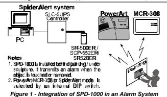
When someone tries to touch or remove the secured object, to which the detector is attached, an identifiable alarm signal is transmitted to alert security personnel. Identifiable signals include: low battery voltage alert, low severity alarm (slight touch) and high severity alarm (repetitive touch, strong touch or In addition, the detector periodically sends supervision signal as a serviceability report. With PowerArt high level, sensitivity can be extended.
