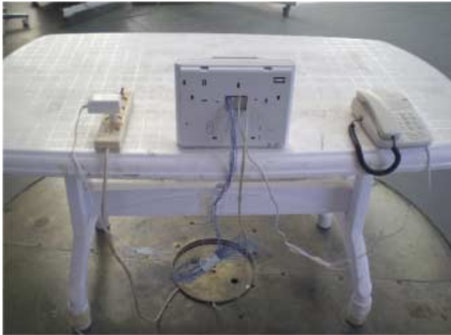
Photograph No.10 Setup for radiated emission measurements at OATS, close view
