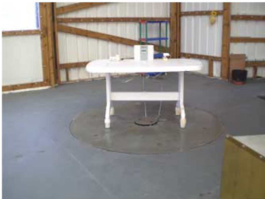
Photograph No.9 Setup for radiated emission measurements at OATS Hz
