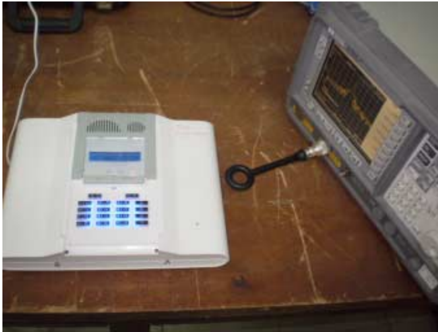
Photograph No.6 Setup for occupied bandwidth test
