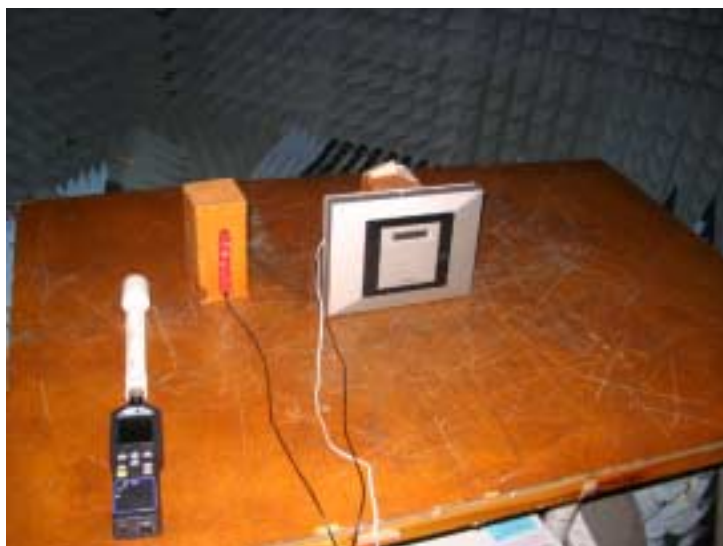
Photograph 7.2.2 Maximum permissible exposure (MPE) measurement set up, EUT with external antenna
