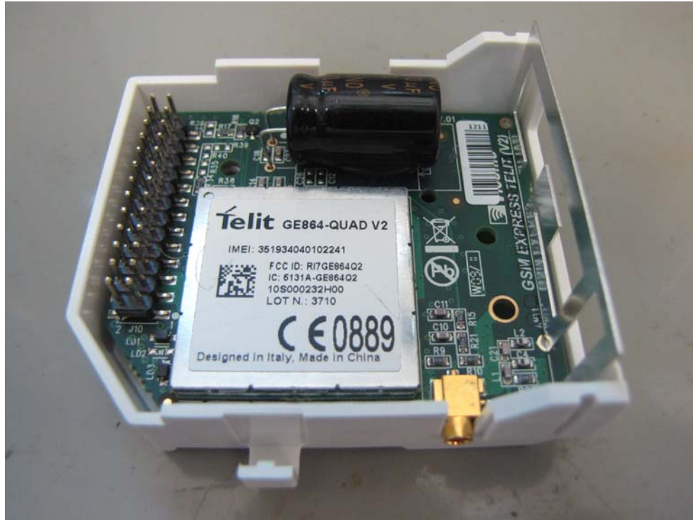
Photograph No.6 GSM modem rear side view
