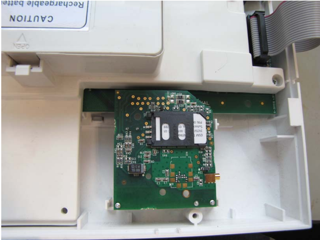
Photograph No.3 PowerMax Pro internal view with GSM modem cover removed
