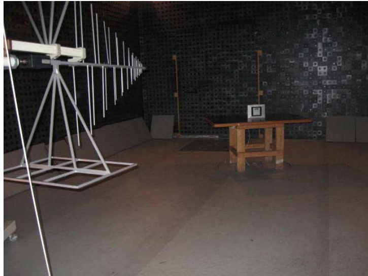
Photograph 7.3.1 Occupied bandwidth test setup
