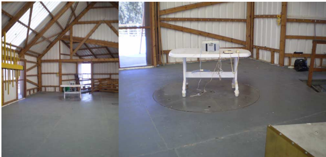
Photograph 8.2.2 Setup for final radiated emission measurements, general view
