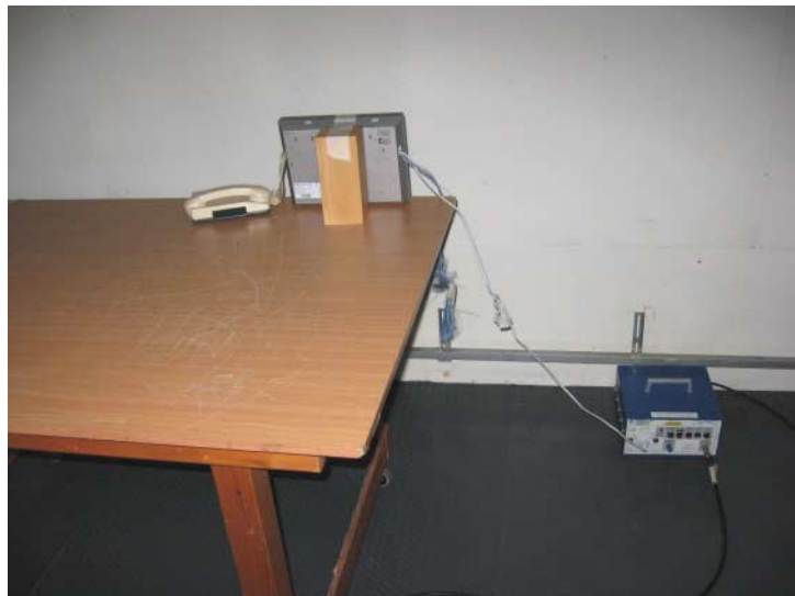
Photograph 8.1.1 Setup for conducted emission measurements
