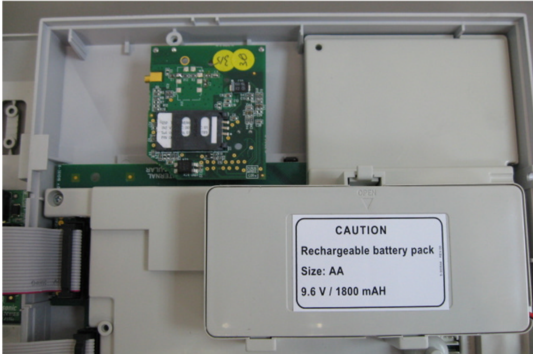
Photograph No.3 PowerMax Pro internal view with GSM modem cover removed
