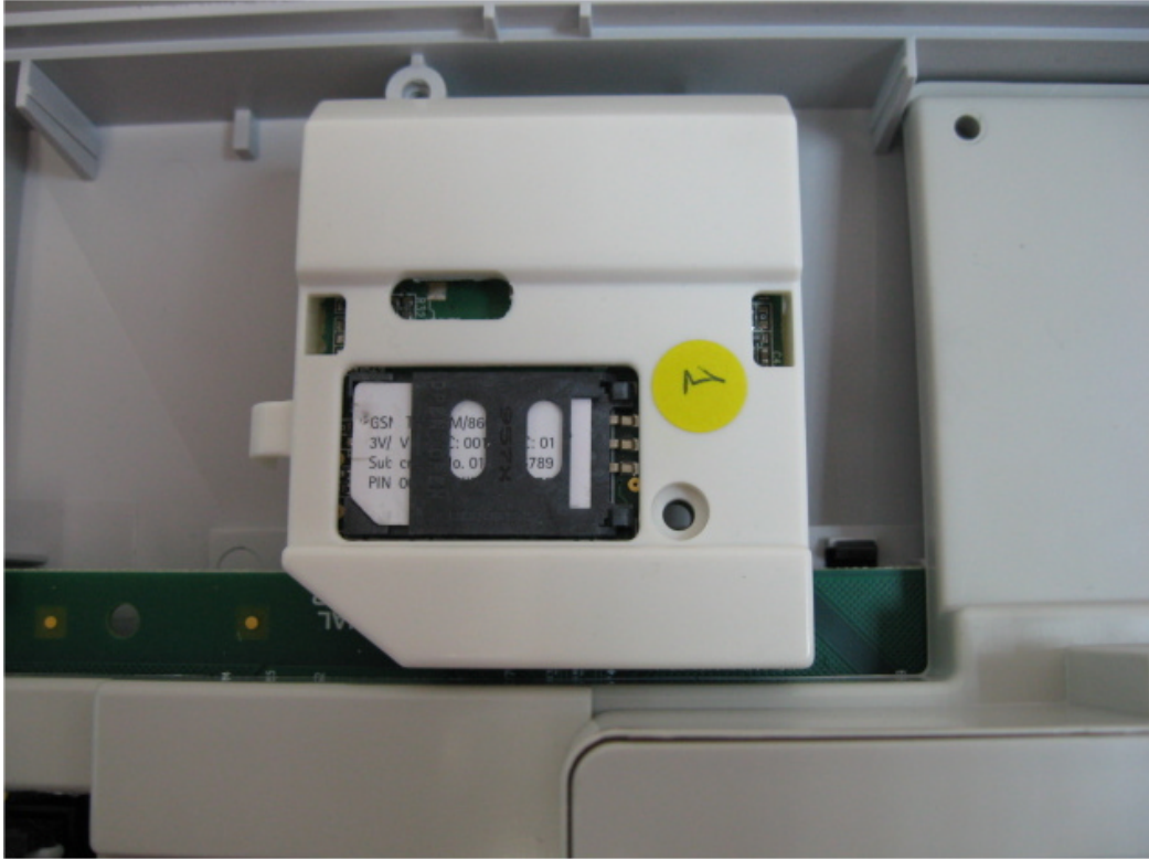
Photograph No.2 PowerMax Pro GSM modem view
