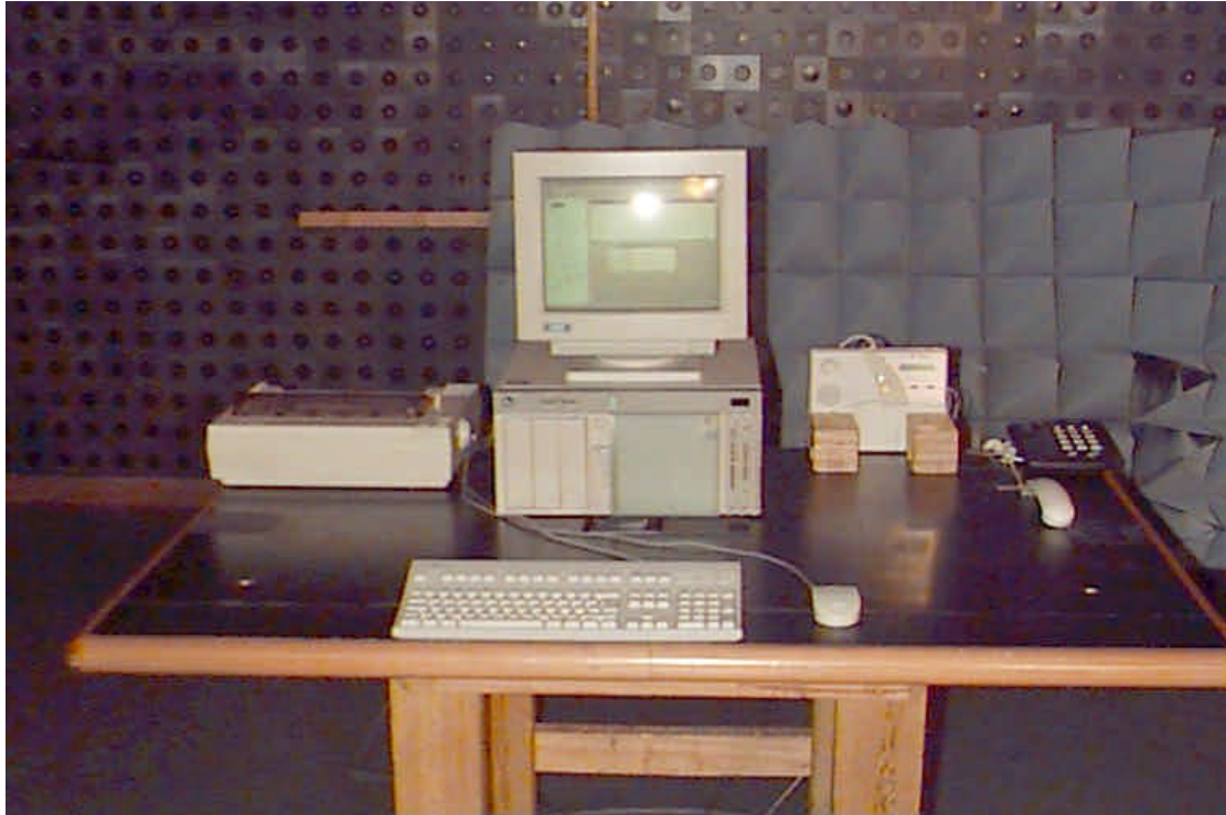
Photograph No.4 Radiated emissions measurement setup in the anechoic chamber
