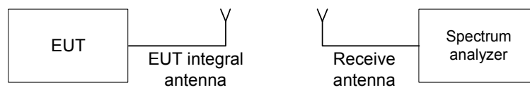
Figure 7.1.1 Setup for transmitter shut down test
