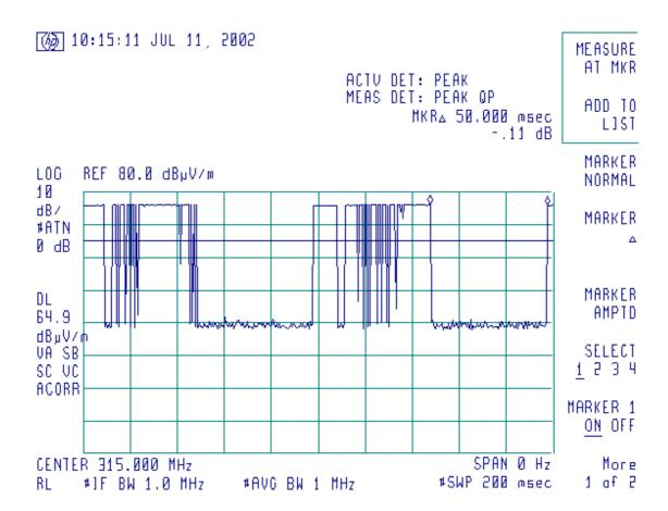
The time between the end of one transmission and the beginning of the other one is 50 ms.
