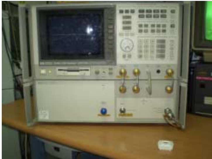
Photograph No.5 Setup for occupied bandwidth test
