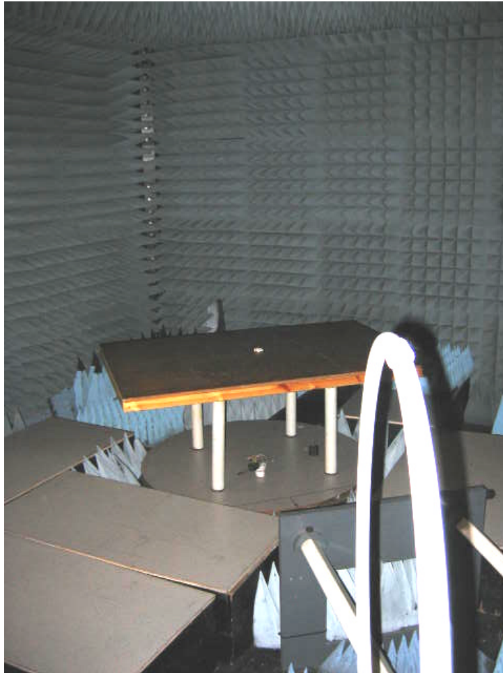
Photograph No.1 Setup for spurious emission field strength measurements in anechoic chamber below 30 MHz
