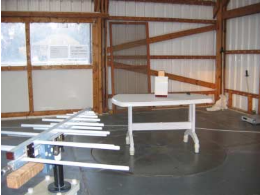
Photograph No.4 Radiated emissions measurement setup at the OATS with log periodic antenna
