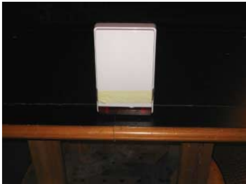
Photograph No.3 Radiated emissions measurement setup in the anechoic chamber, close view
