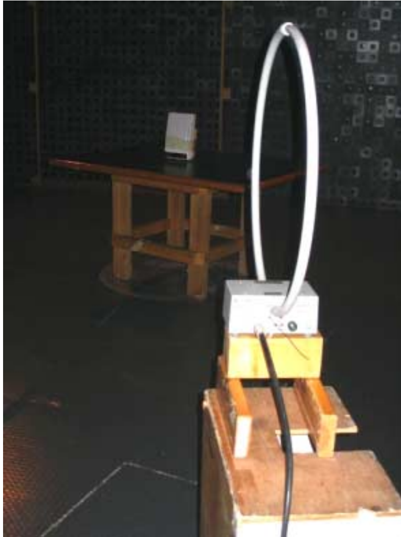
Photograph No.1 Spurious radiated emissions measurement setup in the anechoic chamber with loop antenna
