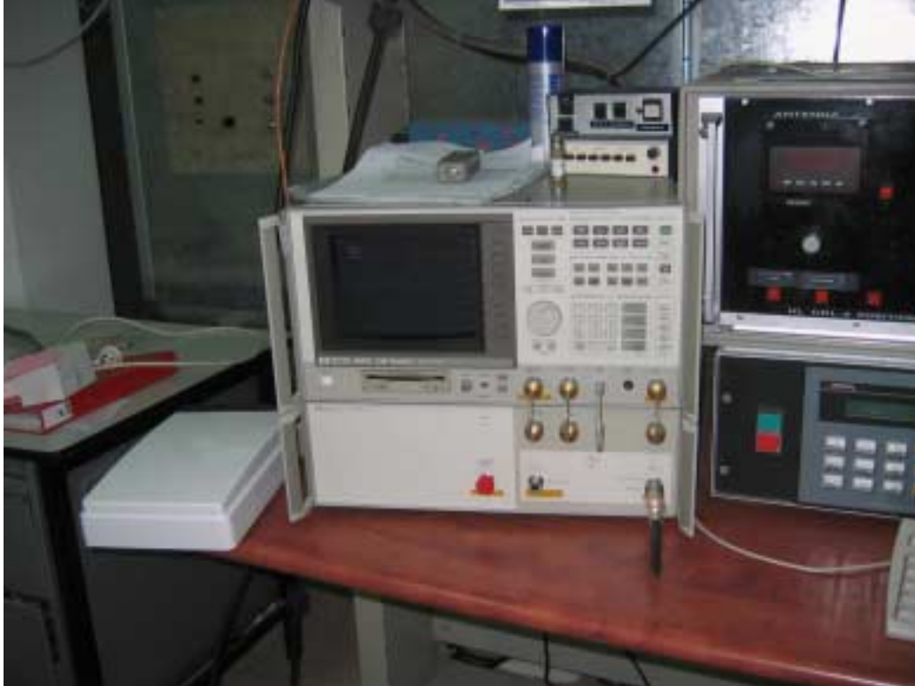
Photograph No.5 Occupied bandwidth measurement setup
