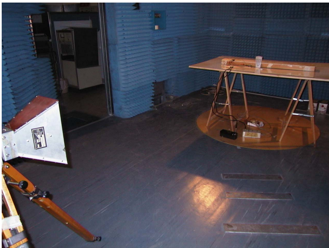
Picture RE/3 Radiated Emission Setup 1GHz-3.5GHz
