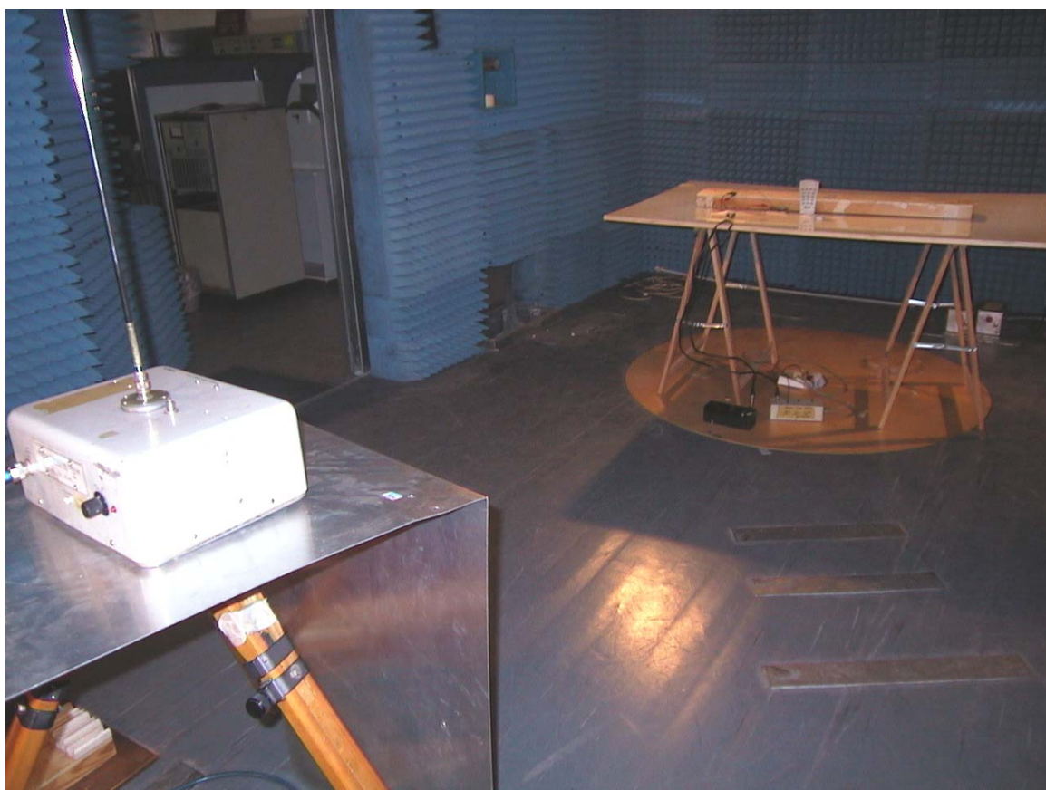
Picture RE/2 Radiated Emission Setup 9KHz-30MHz
