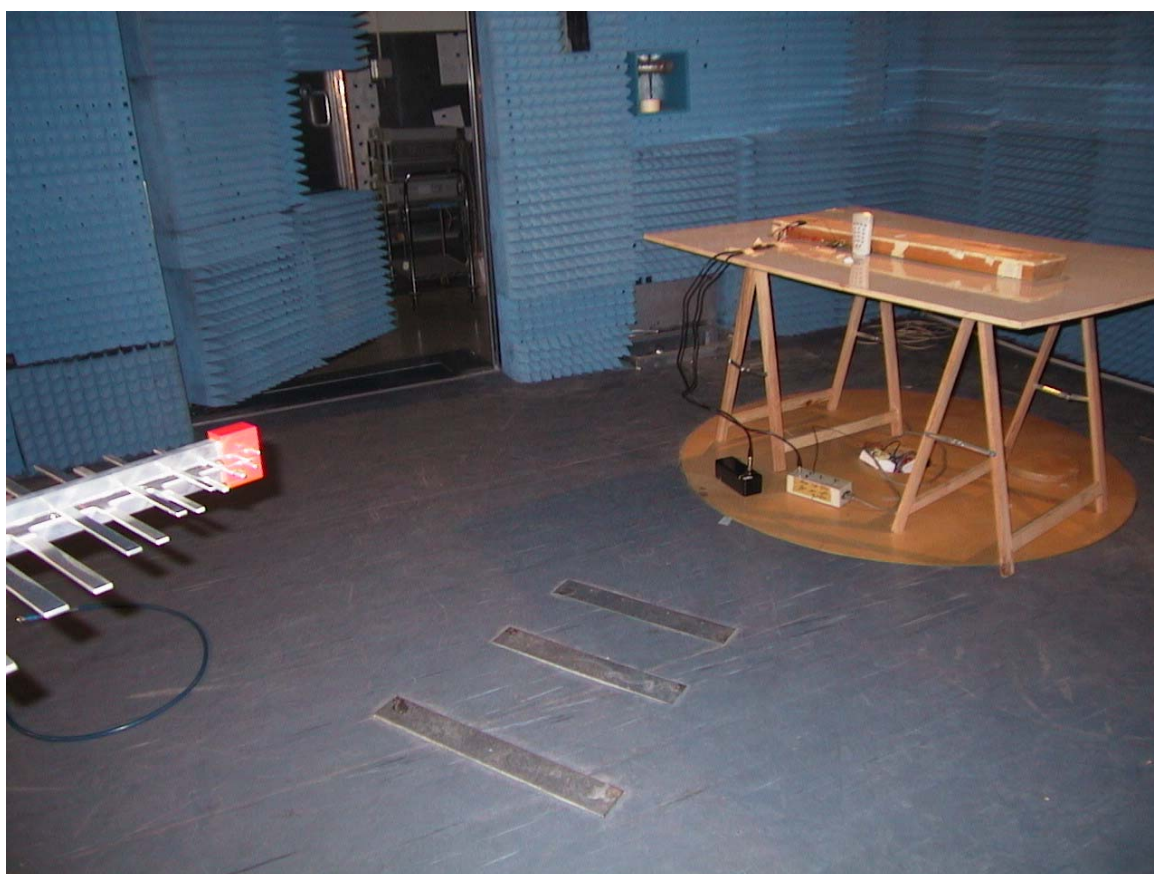
Picture RE/3 Radiated Emission Setup 30MHz-1000MHz
