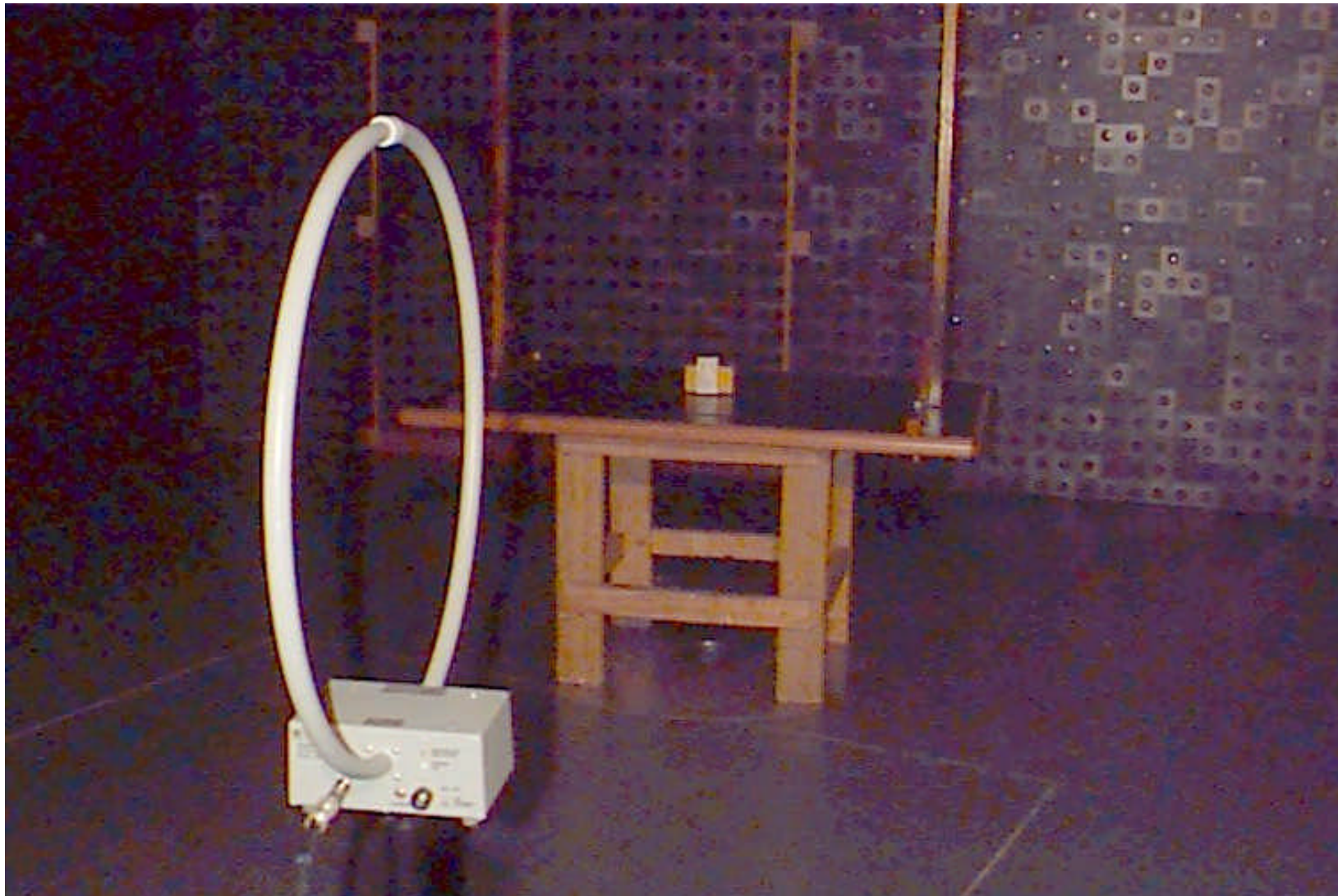
Test setup with loop antenna
