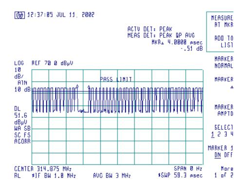
The time between the end of one transmission and the beginning of the other one is 4 ms.
