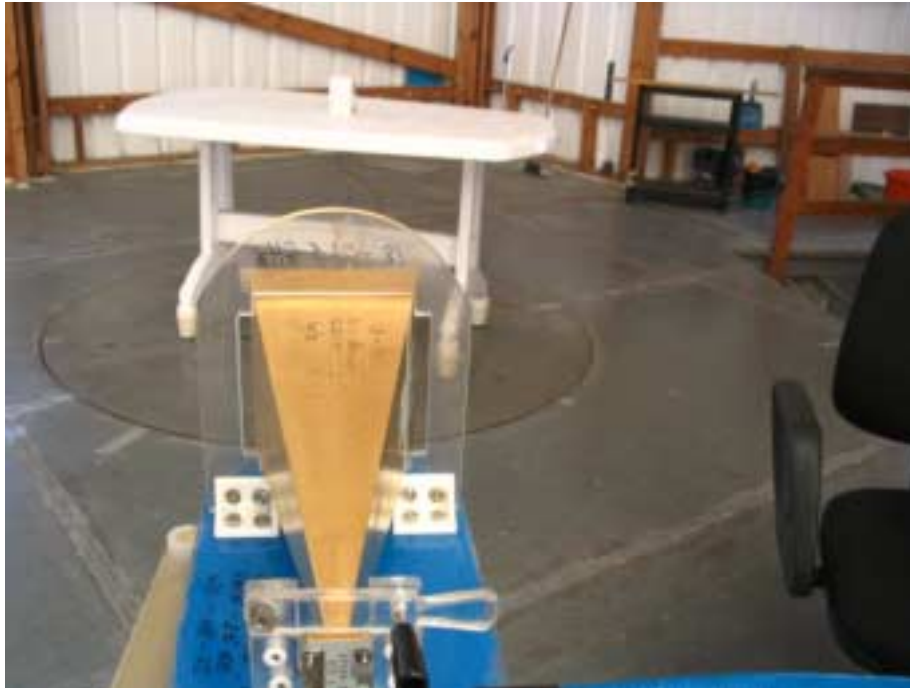
Photograph No.4 Setup for spurious emission field strength measurements at the OATS from 18 to 26.5 GHz
