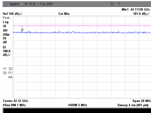
Plot 7.1.20 Radiated emission measurements at the forth harmonic frequency
