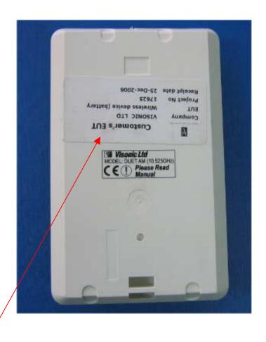
Label with **FCC ID:GSADUETAM** and **IC:1467C-DUETAM** will be located at the rear side panel
